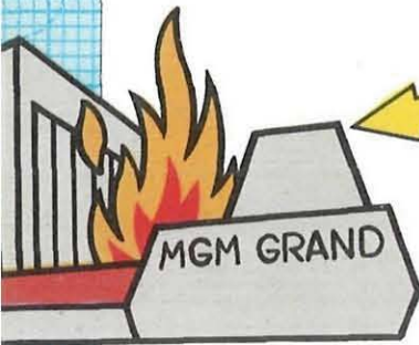
10 Fire reaches decorative false ceiling of flammable foam and sweeps through wind tunnel between false and real ceilings so that entire building instantly bursts into flame!
